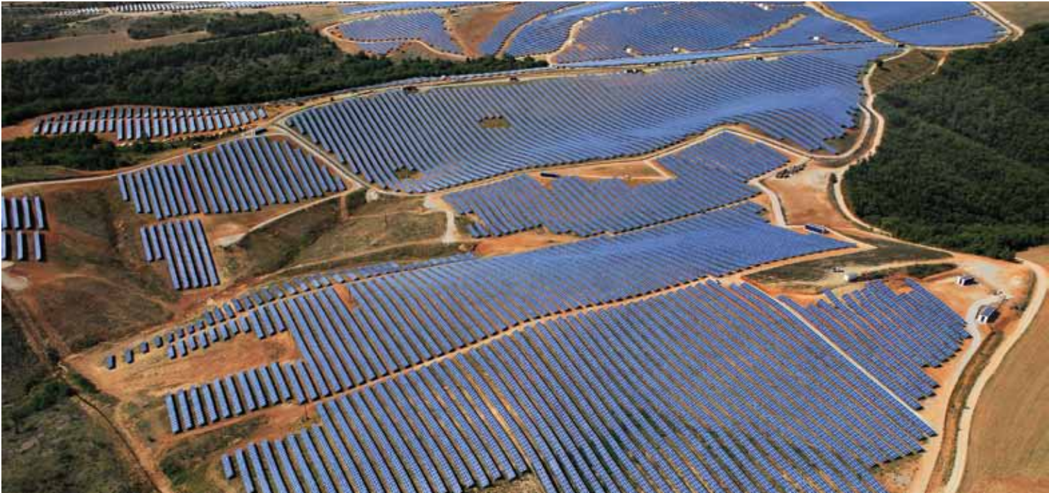
The solar park in Les Mées, France, 31 MWp, provides electricity for more than 12,000 households.
