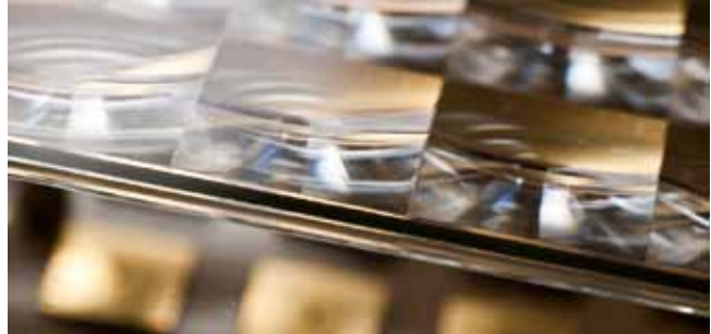
Concentrator systems: lenses to focus sunlight onto solar cells
