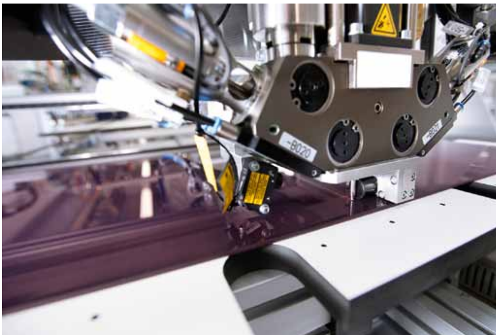
Applying metal contacts to a thin-film module using adhesive
