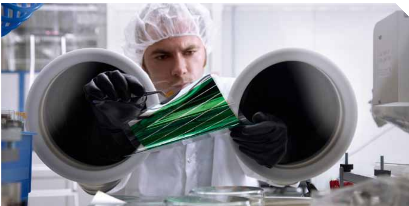
Organic solar cells: preparing a sample in an inert gas atmosphere
