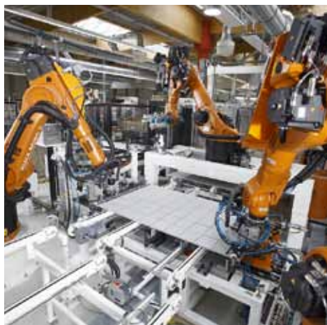
KUKA Systems Robo X – cross-tie soldering
