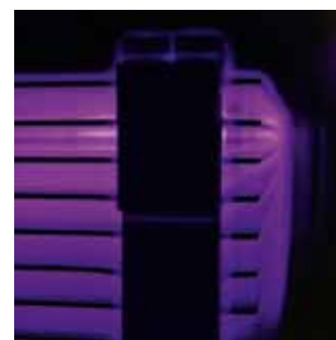
Direct plasma coating: an antireflective coating is applied to cells.
