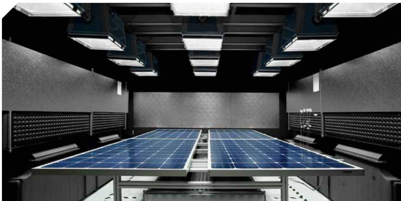
Light aging test on crystalline modules
