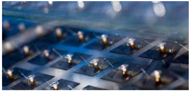
Multijunction cells are produced for use in concentrator systems.
