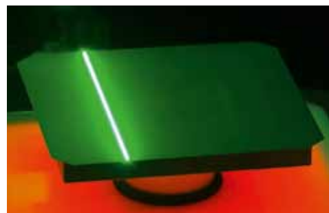
CVD process: doping by means of laser irradiation
