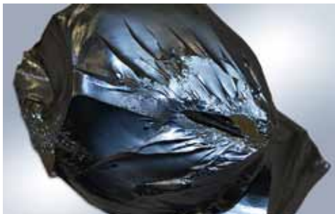
Polysilicon 11N grade produced using the SST monosilane method
