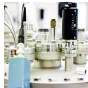
Manufacturing organic solar cells in a vacuum chamber
