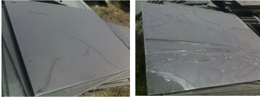
Figure 4.4 Micro-cracks resulting into major cracks in thin film modules
